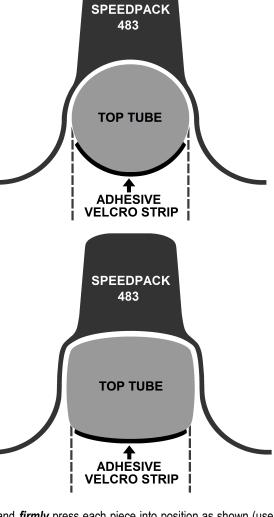
velcro strips without touching the glue and *firmly* press each piece into position as shown (use your temporary tape marks for guidance). After applying the stick-on strips, press firmly on each of them with a roller, or roll over them with a hard round but *non-metal* object (like the round end of a sharpie pen, or the round end of a plastic tool or utensil handle). Firmly pressing the stick-on velcro strips will develop better adhesive contact and will increase their final bond strength.
