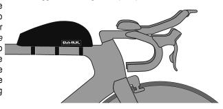
PLACEMENT OF THE ADHESIVE VELCRO: After testing the Speedpack 915's fit in your desired location, before applying the stick-on velcro strips, temporarily mount the Speedpack on your bike and wrap the pack's velcro straps around the top tube. Next, temporarily mark the 3 proposed strap locations on your top tube. We suggest doing this with 6 small pieces of removable colored or masking tape placed on the underside of your top tube as shown. Each of
