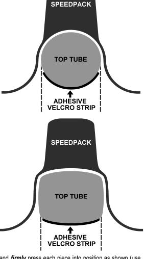
velcro strips without touching the glue and *firmly* press each piece into position as shown (use your temporary tape marks for guidance). After applying the stick-on strips, press firmly on each of them with a roller, or roll over them with a hard round but *non-metal* object (like the round end of a sharpie pen, or the round end of a plastic tool or utensil handle). Firmly pressing the stick-on velcro strips will develop better adhesive contact and will increase their final bond strength.
